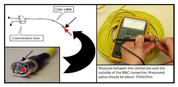
If you measure another value unsolder the detection loop wires from the connection box replace the connection box with coax cable. Measure the detection loop before resoldering.
