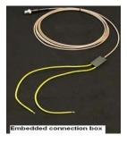
The coax cable and 2 short loop wires are sealed into the connection box
