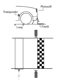
When the hardware system is set up properly, the detection loop is located before the actual finish line, in that way that the transponder is in the middle of the detection loop when the front of the vehicle is crossing the finish line.
