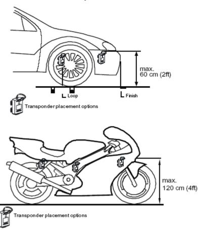
The figure above shows the recommended transponder positions and their maximum heights. Since the transponder signal is limited in strength a maximum mounting height should be obeyed. Higher transponder positions (or positions blocking the signal) will dramatically reduce the received signal strength.
