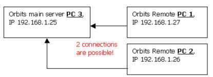
Setup of 1 Orbits main program and 2x Orbits Remote programs
