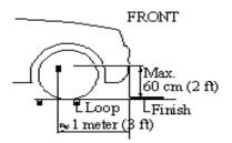
**Step 1** > The detection loop must be positioned in such a way that the transponder is above the center of the detection loop when the front of the cars/motorcycle crosses the finish line. Make sure cars/motorcycle cannot pass outside the detection loop. Extend the detection loop outside the track if necessary.
