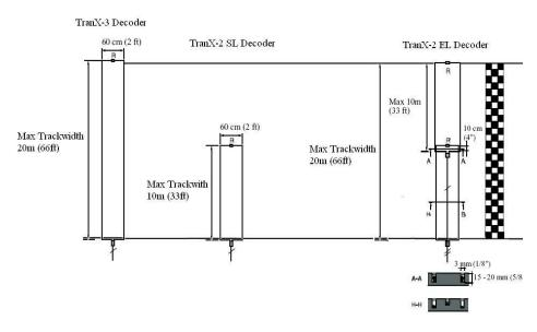
**Step 3** > With a separate loop installed in the pit lane, connect it to the BNC connector marked loop 3 (PIT) on the decoder. Passings registered in the pit lane will be identified as such by the decoder.
