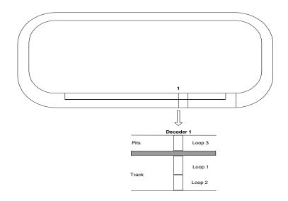
Connecting detection loops to TranX2 Extended Loop Decoder The detection loops are connected to the connectors at the back of the decoder.
