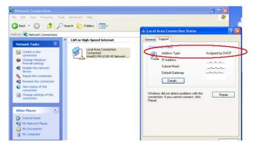
Adress Type within the Support section (see 1) displays how the IP Address is assigned.
