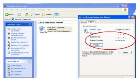
The Support section will display the IP Settings (IP Address, Subnet Mask and Default Gateway)
