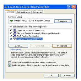
The screen should look like the dialog below with the option "Obtain an IP address automatically" selected
